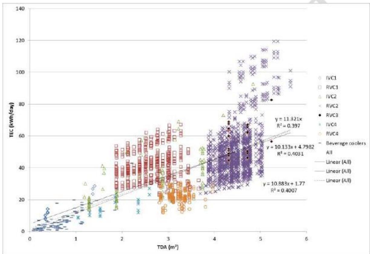
Chart 1 : Cloud of data points for semi-vertical, vertical and vertical roll-in chiller display cabinets and beverage coolers
