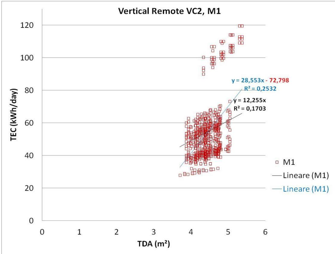
Chart 2 : Segmented data points for vertical chiller display cabinets in temperature class M1
