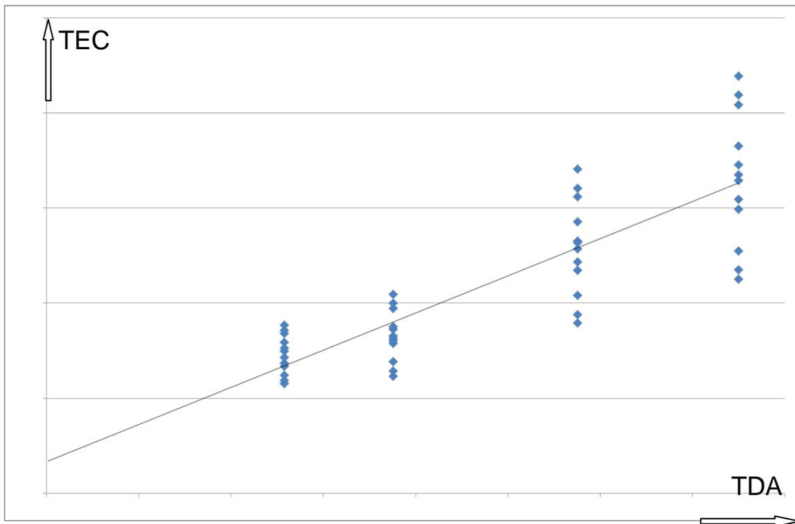
Chart 4 : Segmented data points for vertical chiller display cabinets with different fittings and accessories
