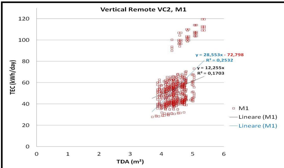
Chart 6 : Segmented data points for remote vertical chiller display cabinets in temperature class M1
