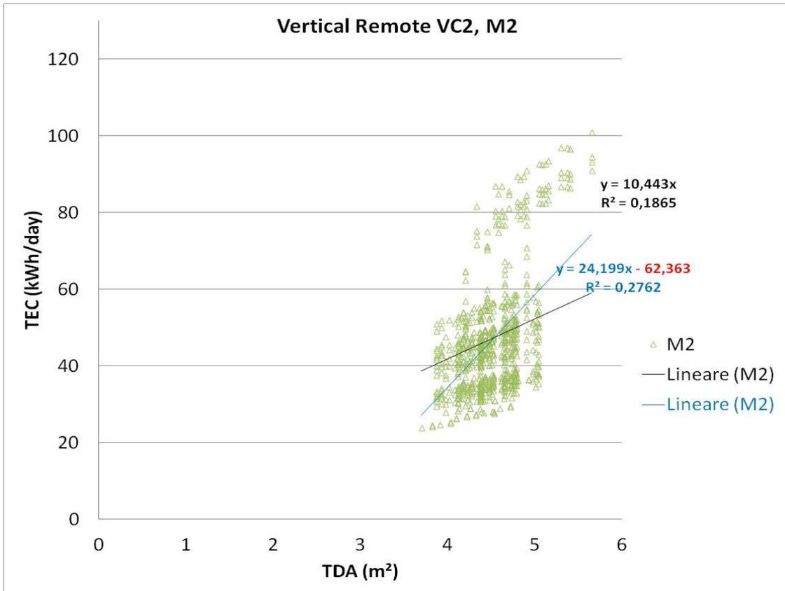
Chart 3 : Segmented data points for vertical chiller display cabinets in temperature class M2
