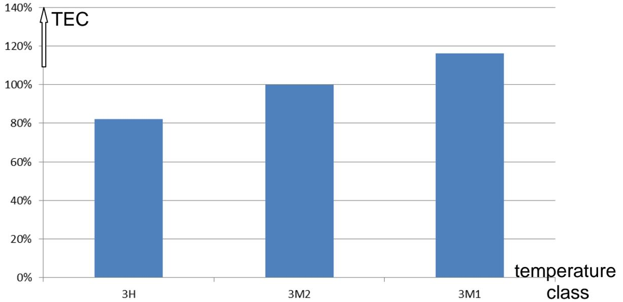
Chart 5 : Comparison of comparable vertical chiller display cabinet models in different temperature classes
